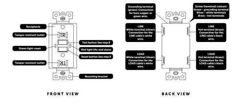
Maximum tightening torque 14in-lbf(1.6N.m)
