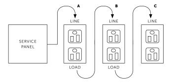
Placing the GFCI in position A will also provide protection to "load side" receptacles/outlets B and C. On the other hand, placing the GFCI in position C will not provide protection to receptacles/outlets A or B. Remember that receptacles/outlets A, B and C can be in different rooms.
