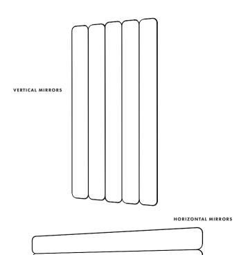
PLACE THE BRACKETS MIN. 40 CM APART. PLACE THE BRACKETS HORIZONTAL IF THE MIRROR SHOULD HANG VERTICAL OR PLACE THE BRACKETS VERTICAL IF THE MIRROR SHOULD HANG HORIZONTAL.
