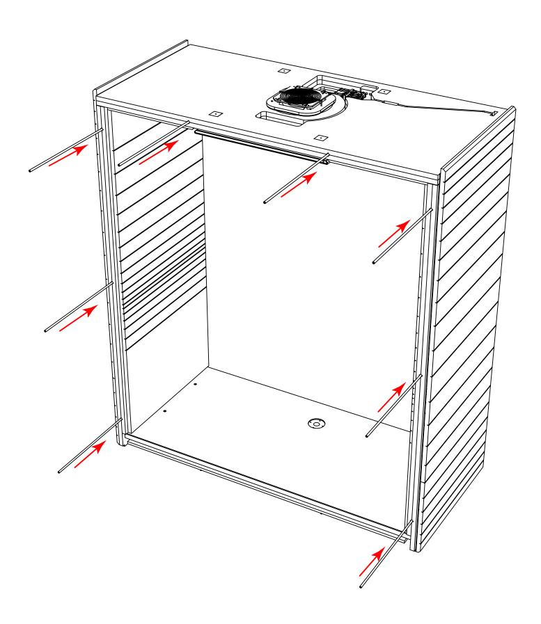
$\begin{array}{c} \text{Step 4} \\ \text{Insert the wooden dowels into the holes. Join the two back panel elements and pull them together} \end{array}$ with the connectors. Do the same with the front elements.
