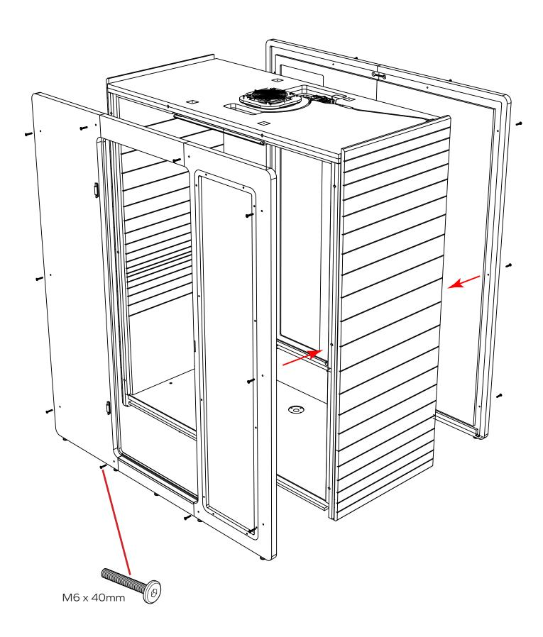
Glue the two 24mm Archisonic panels to the right side of the back panel and the left side of the front. Remove the release paper of the double-sided tape and apply some additional glue dots with the installation glue provided. Make sure that the panels are completely flush with the top and side
