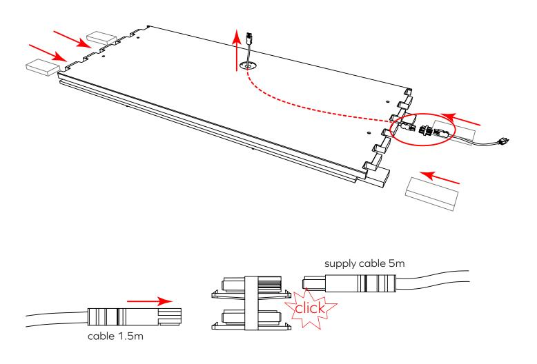
Insert the cable of the right side into the H-distributor. Place the two sides on the honeycomb blocks and tuck them into the bottom. This should go easily, if not, make sure the sides and bottom are aligned. Hold the sides until the top is assembled. Pin the top together with the sides, pull the cable through the top from the right side.
