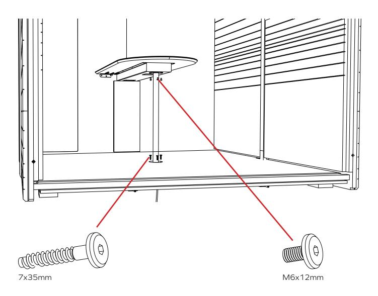
Connect the table top to the back wall with six 7x35mm screws. Screw the benches onto the floor with the 7x35mm screws. Carefully loosen the cover of the socket. Connect the socket with the supply cable. Insert the socket into the hole. Align it and tighten it. Place the insert and snap the cover back into place.
