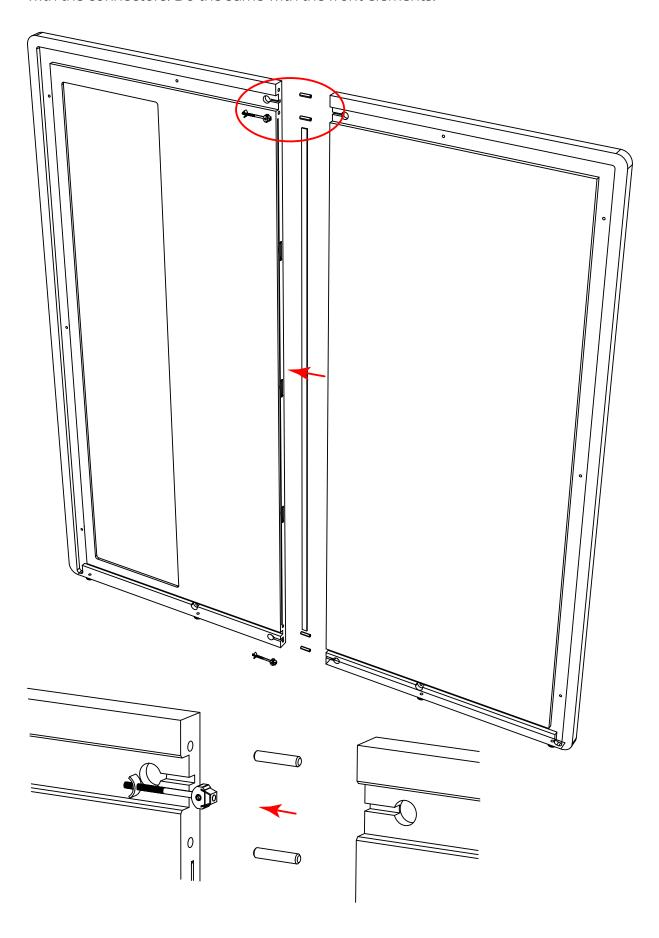
$\begin{array}{c} \text{\bf step 5} \\ \text{\bf Join the back wall with the sides, the bottom and the top. Secure the back panel by screwing the} \end{array}$ six screws a few turns into the connecting rods. Do the same with the front. Now tighten all the screws, which must be countered on the opposite side.
