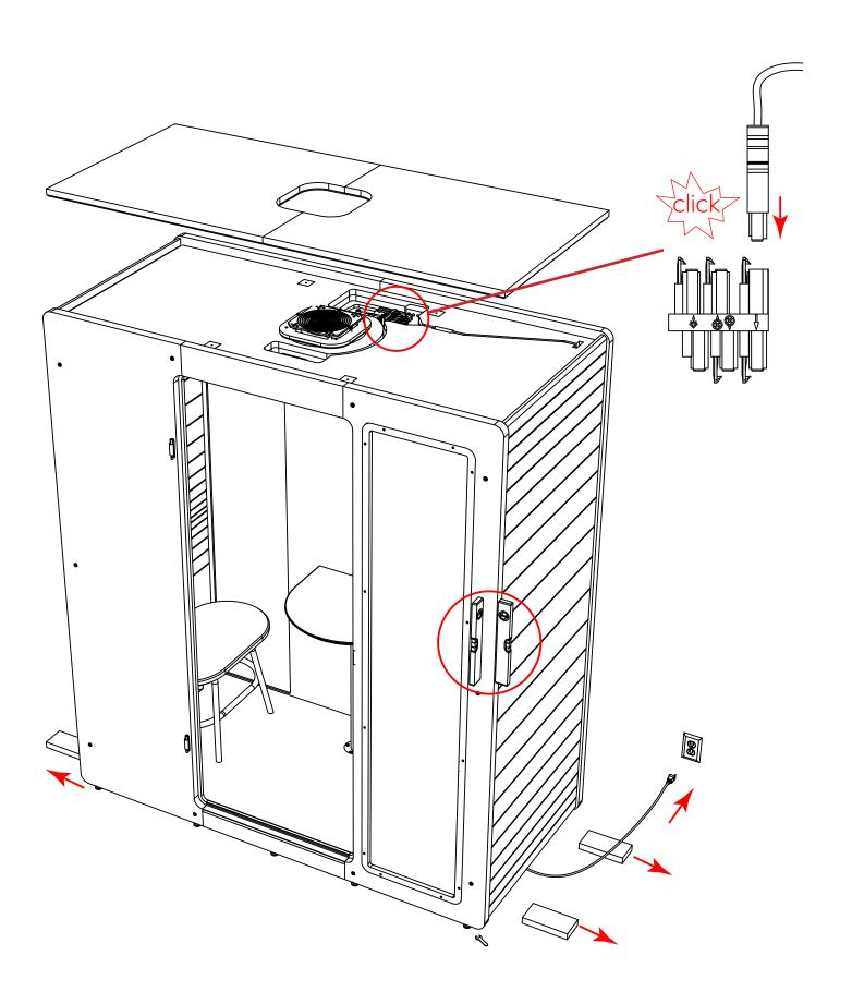
Mount the door and fix it with the two rods. Secure them with the set screws. Assemble the door handle in the following order: lock, metal washer, plastic washer, door handle. Press the two halves of the door handle together while tightening the stud screw with the 3 mm hex key. Make sure that the handle is mounted with the pre-mounted square pin in the inside of the chatpod.
