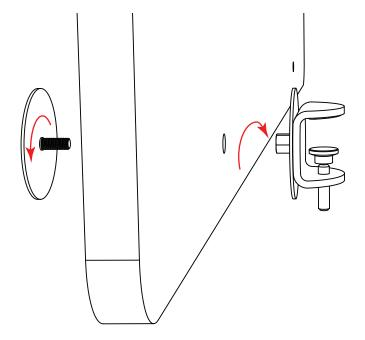
**2.** Clamp the adapters to the desk top with the clamping screws.
