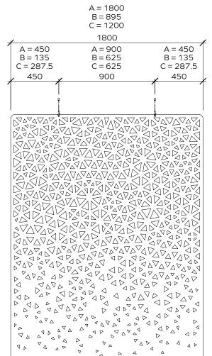
The screws for fixing to the ceiling are not supplied. Either an M6 set screw, a M6 hanger bolt or a wood chipboard screw with a maximum diameter of 5mm can be used.
