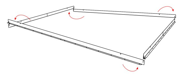
$\begin{array}{c} \text{Step 2} \\ \text{Fasten the frame in the center with the included screws. Tighten the screws only slightly.} \end{array}$
