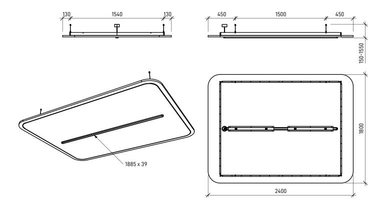
$\begin{array}{c} \text{Step 1} \\ \text{The four frame elements are joined together as shown.} \end{array}$
