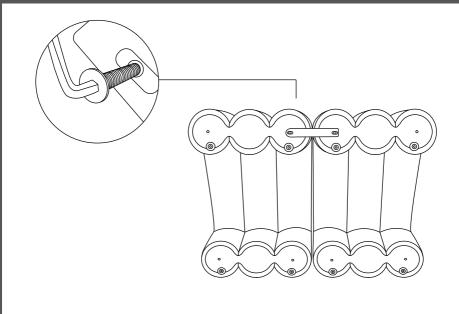
3. Align the bracket so that the screw hole is visible through the hole in the brackets. Utilize the allen key to secure the screw into the chair. Repeat this process on the corresponding chair.
