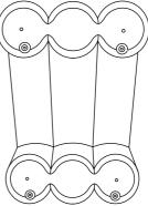
2. Place the chairs side by side and gently tilt them backward until they rest on the back legs. Locate two holes beneath the front legs and two holes beneath the back legs. It is advisable to have at least two people present during the assembly process.
