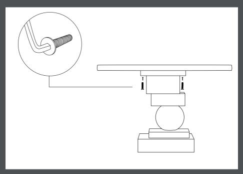
3. Once aligned, insert and align the four screws to secure the installation.
