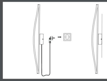
Plug the socket into a power outlet. If there is a built in lamp socket in the wall, the lamp can also be mounted directly to the wall without the cable.
