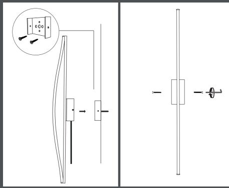
1. Detach the mounting plate from the wall lamp and mount it to the wall. Make sure to use appropriate screws and rawlplugs/anchors. Mount the wall lamp to the plate on the wall using the plated screws. Turn the screws clockwise for fastening.
